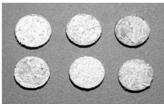
Figure 4. Tablets for investigation of ash content, sulphur and high calorific value of briquettes made from different raw material.
