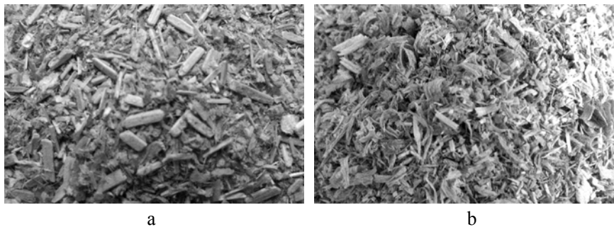
Figure 3. Chipped raw material for production of briquettes. a - tobacco stems, b - beech wood.
